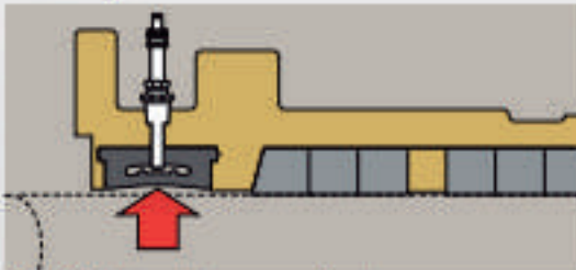
The Air Seal ring in original concave configuration
